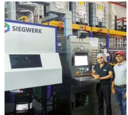
The new automated ink dispensing system reduces ink dispensing time by 68 percent.
